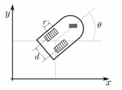
$$\begin{cases} \dot{x} = \frac{\omega_R + \omega_L}{2} r \cos(\theta) \\ \dot{y} = \frac{\omega_R + \omega_L}{2} r \sin(\theta) \\ \dot{\theta} = \frac{\omega_R - \omega_L}{d} r \end{cases}$$
